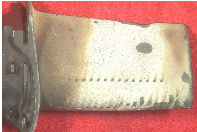
Exposure of turbine blade by erosion.
