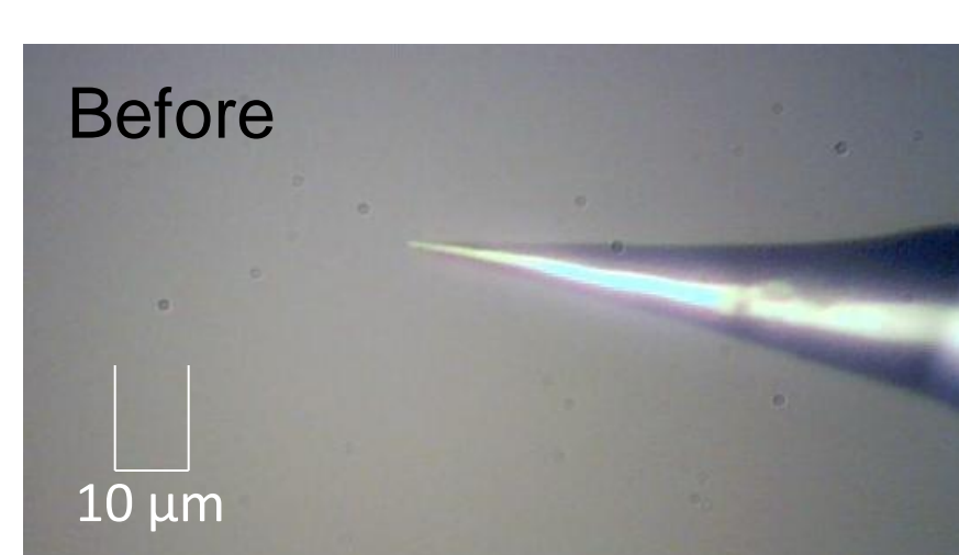
Future tip preparation techniques include surface roughening via chemical etching, as shown above.
