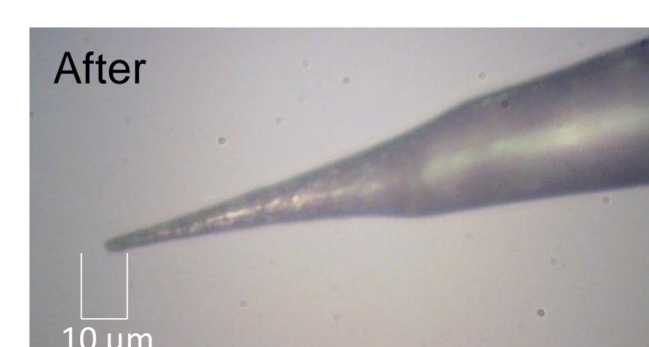
Future tip preparation techniques include surface roughening via chemical etching, as shown above.
