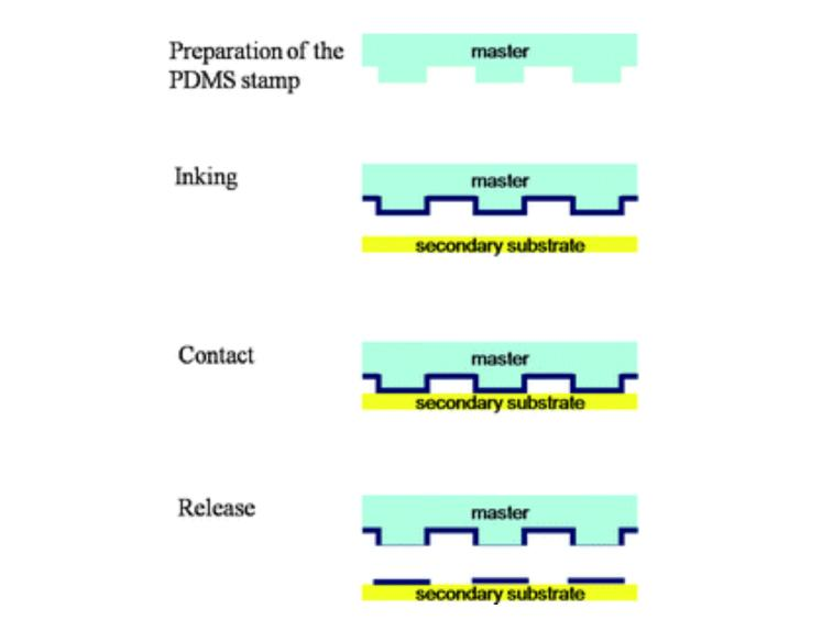
The pillar geometries on the PDMS stamp are treated with Aminopropyltriethoxysilane (APTES) to make the stamping surface more hydrophilic. Then PLL is deposited onto the treated surface.
